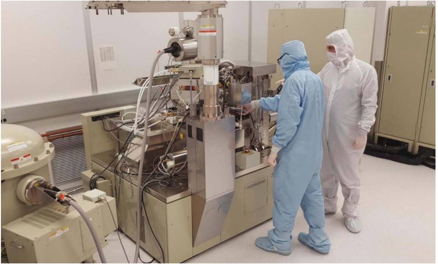
Figure 4: Nano-fabrication scientists set up Authenticity EBL system inside a Class-100 cleanroom
